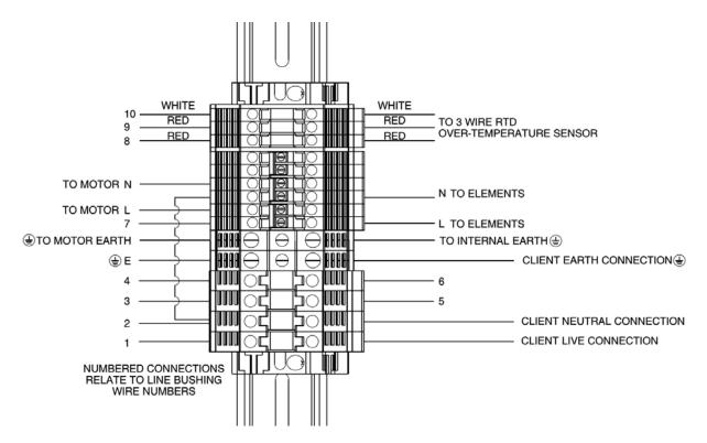
Fig. 12.2 Single Phase Ex e enclosure, terminal wiring Diagram. Connections to be made in accordance section 5 of this IOM.
