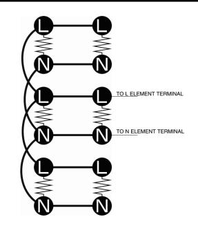
Fig. 12.1 Single Phase element wiring Diagram.
