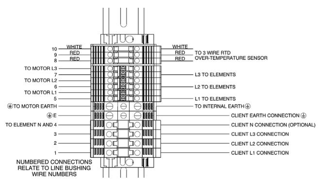
Fig. 12.4 Three Phase Ex e enclosure, terminal wiring Diagram. Connections to be made in accordance section 5 of this IOM.
