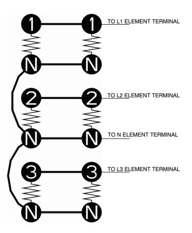
Fig. 12.3 Three Phase element wiring Diagram.
