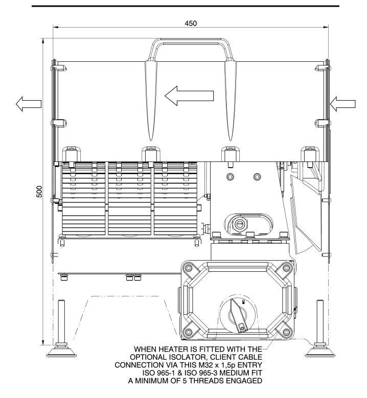
Fig 11.1 General arrangement drawing for both T3 and T4 MFH heaters when fitted with the optional local isolator.
