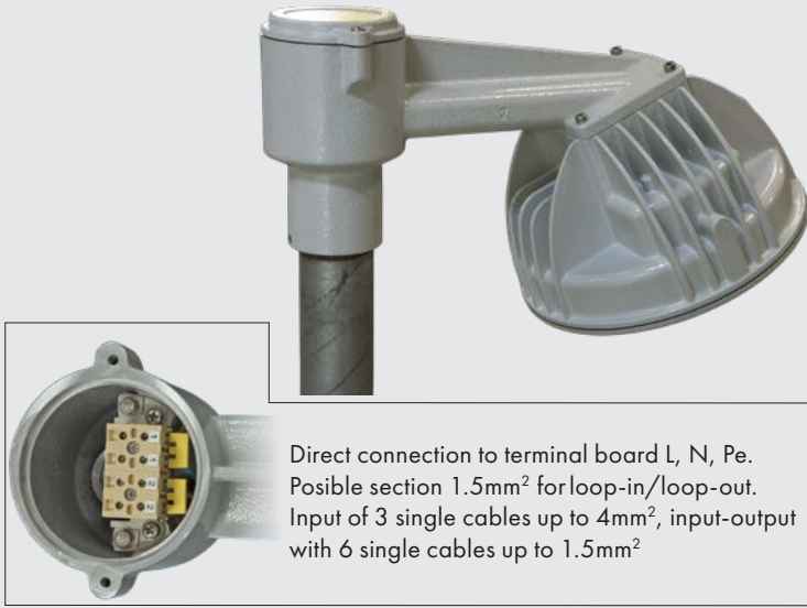
Stanchion mounting with fixed orientation at 25°
