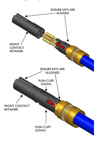
19) Slide the insert into the connector body, aligning the half round key on the rear contact retainer with the required half round keyway in the connector body. (The colour coded or numbered keying position is shown on the front of the connector body. No colour coding or numbering for default 12 o'clock position – see picture inset). It should be noted that colour coded and numbered connector bodies are mutually interchangeable. Push the octagonal portion of the spigot into the connector body.
