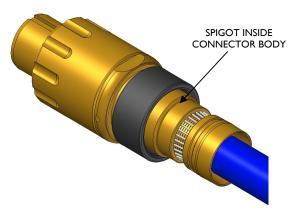
20) Slide the middle nut over the clamp / spigot and hand tighten onto the connector body, then further tighten ½ to ¾ of a turn with a spanner while holding the front shell with a spanner
