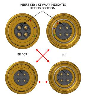
3) Engage the CP connector with the BR / CR connector and align the keyway on the CP connector to the key on the BR / CR connector.
