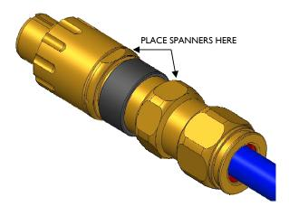
10) Unscrew the middle nut and visually inspect that the armour has been successfully clamped between the armour spigot and the clamping ring.
