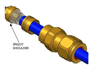
9) Place the connector body over the spigot engaging the octagonal portion of the spigot. Move the middle nut up to meet the connector body. Place a spanner on the flats of the connector body and hold it in position. Hand tighten the middle nut to the connector body, then turn a further ½ to ¾ turn with a spanner.
