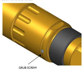
To disconnect, slacken the tightened grub screw, turn the engaging nut anti-clockwise and remove the connector. Fit the caps.
