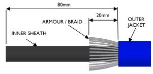
7) Strip back the inner sheath level with the armour to expose the insulated conductors as shown below. If unarmoured, strip back to the outer jacket.
