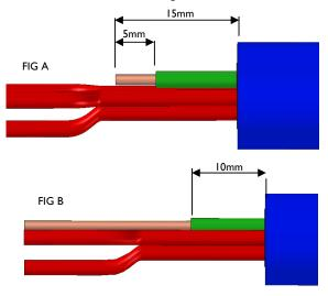
12) Crimp the flat blade earth crimp onto the earth conductor as shown below. Ensure the blade of the crimp is outermost, as shown and that the crimp is pushed all the way up to the insulation of the earth conductor.
