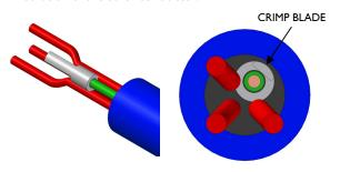
13) Push the conductors through the spigot and place the blade of the crimp on the taper of the spigot.
