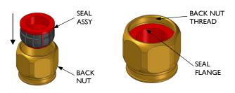
4) Screw the backnut onto the middle nut. Do not compress the seal at this stage.
