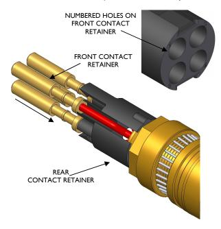
18) Slide the front contact retainer over the contacts and snap into place with the rear contact retainer. Push the clips of the rear contact retainer firmly down to ensure they are not protruding (will only fit in the correct orientation).
